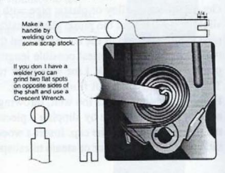
hook of the spring and insert the tool in the center. Turn the tool to compress the spring until it fits into the slot. Release the tool. Tap the spring into position with a hammer.
