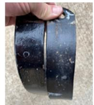
to appear. It is very common to see 1930 or before cars with 1931 bumper arms on them. The edges of the brace are more rounded on the original, and frequently a "C" is cast into them. (Original bumpers also tended to have a "C" cast into them, but not always.) Additionally, the original brace holds the bumper well away from the tires. There should be at least four inches between the tire and the end of the bumper.
