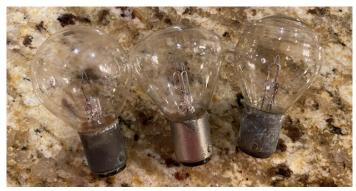
So, which is the original and correct bulb for a Model "A"? The one in the center is a new bulb purchased from Bratton's or some other vendor. The bulb on the left is just an old bulb. I'm sure it would emit light though. The bulb on the far right is the one that is truly special. Can you see the ribs in the glass envelope? That's the type of bulb a Model "A" came with. Additionally, the base was originally nickel-plated brass. It appears as though the nickel is almost gone after 90 years or so.
