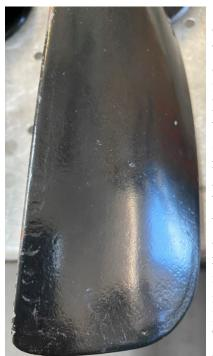
In July 1930, an engineering drawing was released for a single thickness fan produced by Holley. There were two variations of this style. Initially, the new design called for a large radius on the back where the single thickness blade was attached. This large radius was eliminated in late 1930. Below is a photo of the later style radius. This fan was used in conjunction with the
