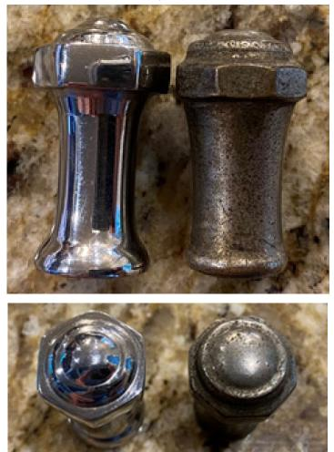
It seems to be a little fuzzy on when Ford actually changed over to produce the 1929 open car body styles; however, by at least December 1928, Ford had replaced the knobs with the new handles for the new 1929 bodies. The new style was used throughout the rest of production with only one change beginning in mid-1930. The handle on top is an original for 1929 through early 1930 that has been restored. As you can see, they were nickel plated whereas the reproduction on bottom is chrome.
