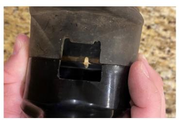
The other difference is the slot in the lower skirt for the locating pin. In 1931, they reduced the height of the opening to approximately 5/64" to lower the possibility of dust entering through this hole. Don't worry! The yellow tape in the below photograph is not original!
