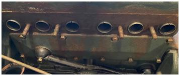
The next photo shows the installed 1928 gaskets. The difference from the 1929 version is easy to spot. On a side note, Dad's January 1929 motor also has this style of gaskets, and he received full credit for them since it's within the two-month rule.
