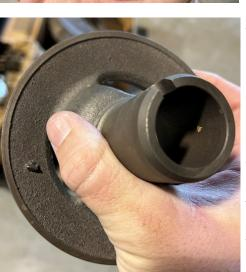
second telltale sign is the casting "delta" on the back side as seen in the second photo. With few exceptions, original Ford castings have a "delta". This crankshaft pulley will be painted Engine green and installed on a 1931 project I am just starting on. Hopefully as I go along, I will have more updates for you all. In the meantime, if you're looking at a cast piece at a swap meet,
