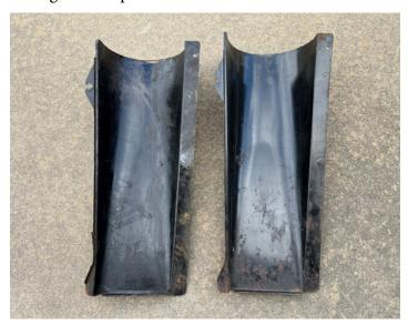
You might be looking at these thinking, "What's the difference?" The one on the right has an extra hole that was only added after June of 1930. This hole was only used on "AA" trucks. Other than that, they are exactly the same. Below is a photo of the extra hole on the NOS pan. Isn't that original paint just gorgeous? I supposed if you were desperate, you could probably find a way to add the extra hole to the one on the left.
