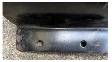
Below is a photo showing the bottom side of the NOS late pan. You can also see the proper shape of the pan from this angle. It is not round all the way to the front like the reproductions are.
