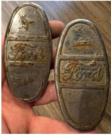
As you can see, the recessed areas are very shallow. When Ford redesigned the early clamps the increased the depth of the recessed area. In the photo at the top of the next column, you can see how much deeper the recess is. The recess was shallow on both the front and rear clamps in early 1928.
